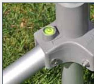
**Level indicator.** Aids a quicker set up and more accurate elevation reading.
